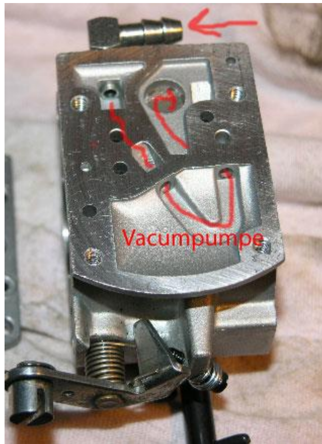
Path of the fuel as it enters the carb.
