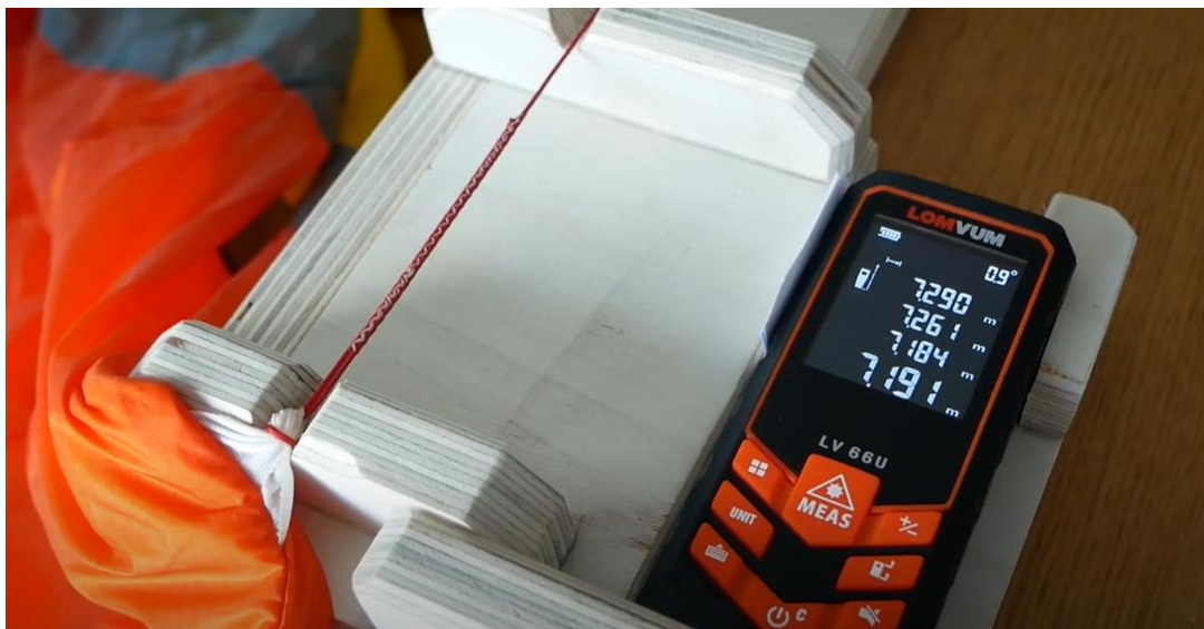
Paraglider Line Tester : Measures the line length, and stretching.
